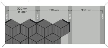
\* The spacing of the battens from a perpendicular wall may vary depending on the desired panel placement and wall length. Please check out our Installation Manual on our website for detailed guidance.
