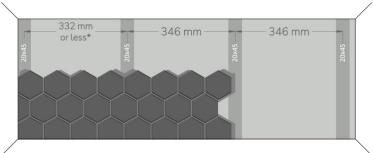
\* The spacing of the battens from a perpendicular wall may vary depending on the desired panel placement and wall length. Please check out our Installation Manual on our website for detailed guidance.
