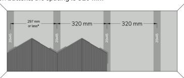
\* The spacing of the battens from a perpendicular wall may vary depending on the desired panel placement and wall length. Please check out our Installation Manual on our website for detailed guidance.
